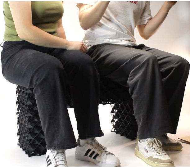
Figure 15: The assembled bench supports two people.
